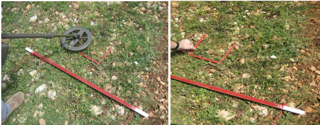
Figures 14 and 15: Example – Marking for detector signal isolation (Photos provided by Doug Ware, UNMAS)
