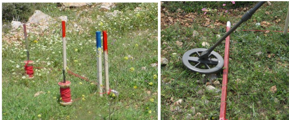
Figures 17 and 18: Example – Bobbins and cord attached to Base Stick (Photos provided by Doug Ware, UNMAS)
